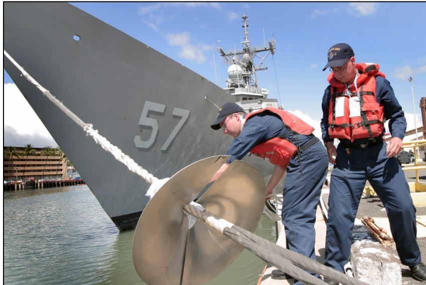
Figure 3-13. Example of a rat guard that should be installed on all vessels at dock travelling to NALF SCI. Source: US Navy.
