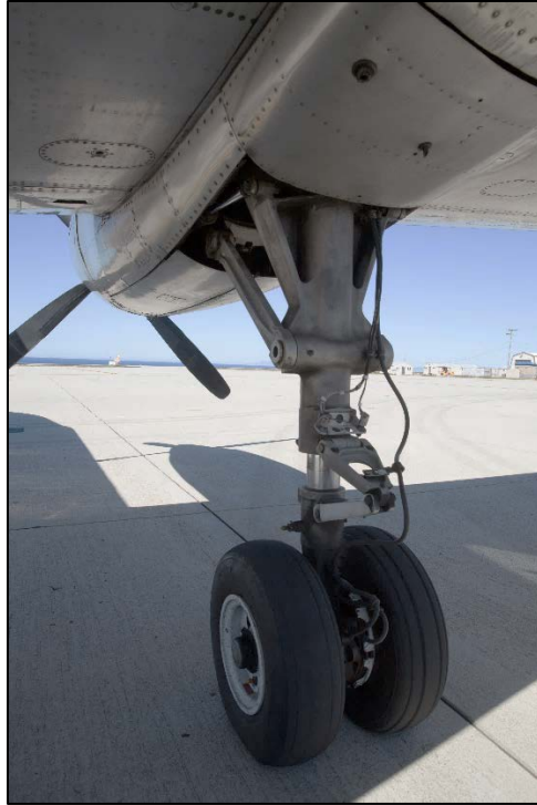
Figure 3-20. Landing gear is easily accessible and may provide refuge for rodents and mesopredators. They should be regularly inspected.
